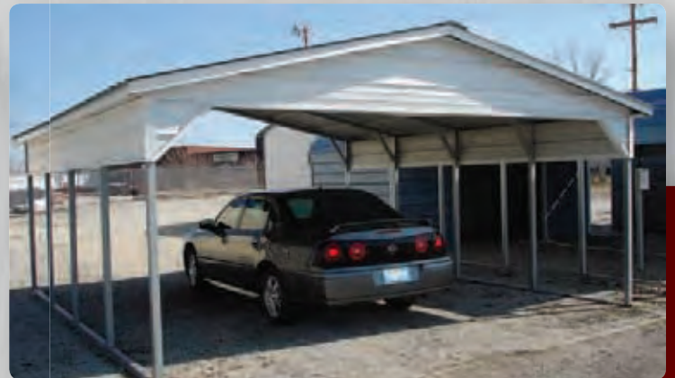
18'W X 21'L X 7'H A-Frame with 1 gable end, 1/2 panels on each side & 45° cuts
